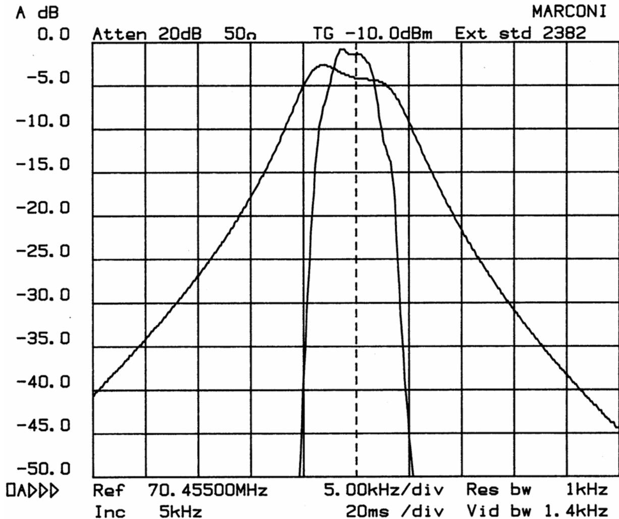
The wider trace is the unmodified RF board response and the narrow trace is after the Inrad mod is installed. There is a small increase in gain that has a slight effect on lowering the noise floor.
